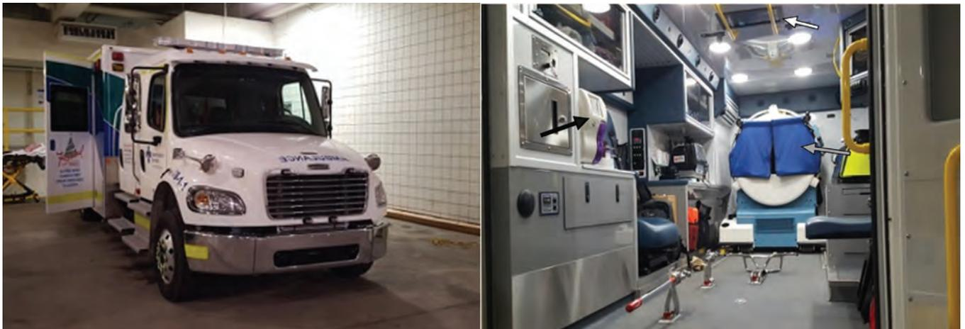
**Figure 1:** The mobile stroke unit based at the University of Alberta Hospital in Edmonton (left photo). The ambulance (right photo) is equipped with a computed tomography scanner (grey arrow), “point-of care” laboratory (analyzer model poch-100i, Sysmex Canada; black arrow) and telemedicine equipment (white arrow).
