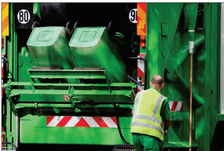
Workers minimize health and safety risks by wearing protective gear and, when available, using a garbage truck's automated loading system for heavy bins.
