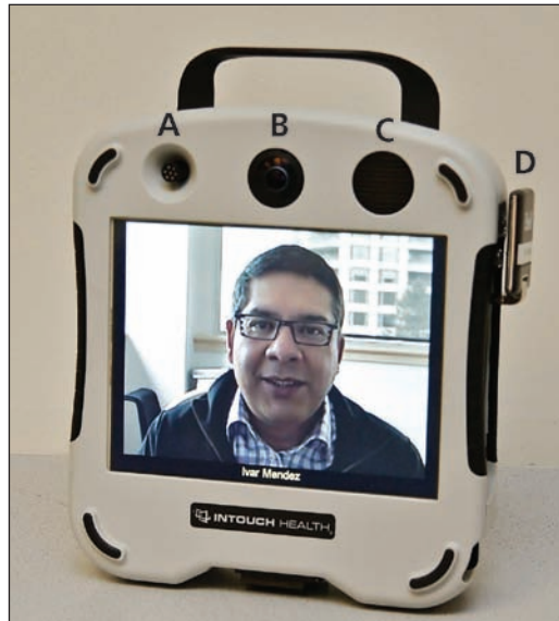
Figure 2: The (A) microphone, (B) high-resolution pan-tilt-zoom camera, (C) high-performance speakers and (D) cellular network modem of the RP-Xpress.
