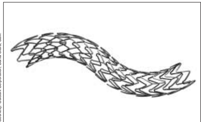
Fig. 3: Stents such as this one (the ACS MULTILINK DUET balloon-expandable coronary stent) are commonly used during percutaneous transluminal coronary angioplasty (PTCA) in Canada. The stent is laser-cut from tubular stainless steel in a design providing radial strength and longitudinal flexibility. Stent diameter is determined by the balloon diameter used for deployment.
