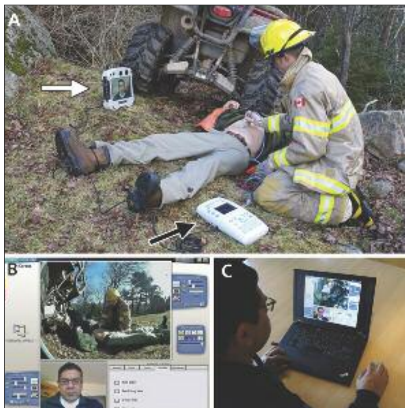
Figure 1: (A) Scene of a simulated accident showing the RP-Xpress (white arrow) and a portable ultrasound machine (black arrow). (B) Image of the screen of the RP-Xpress. This screen has 2 main displays that show the operating physician at the (C) control station, as well as the image of the remote location, allowing for early assessment and diagnosis of an injured person before arrival at the emergency department.
