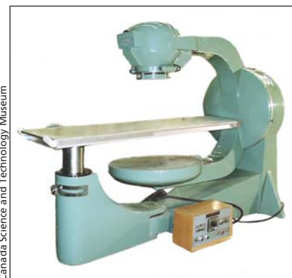
A radiation therapy machine, Theratron Junior, Atomic Energy of Canada Ltd., 1957 (acc. no. 1966.0043).
