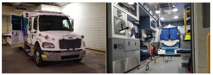
Figure 1: The mobile stroke unit based at the University of Alberta Hospital in Edmonton (left photo). The ambulance (right photo) is equipped with a computed tomography scanner (grey arrow), "point-of care" laboratory (analyzer model pocH-100*i*, Sysmex Canada; black arrow) and telemedicine equipment (white arrow).
